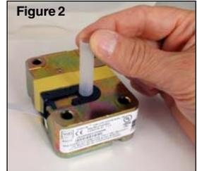
5. Remove lock case assembly from door and cut the tube just inside your mark.
