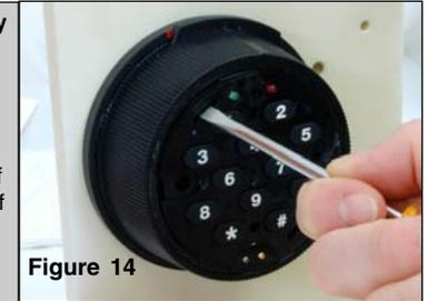
14. If your lock includes the Battery Assist option, you should now mount the battery clip inside the door near the lock and install a fresh 9 Volt Alkaline battery.
