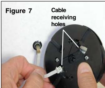
3. Align the dial assembly with the mounting holes and spindle, and position against the outside of the container door.
