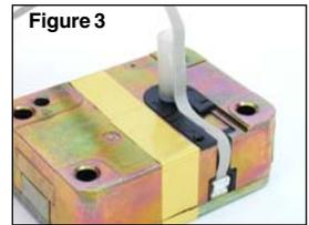
8. Hold the lock case assembly and carefully guide the loose end of the ribbon cable and the tube through the spindle hole so that they are accessible outside of the container door.
