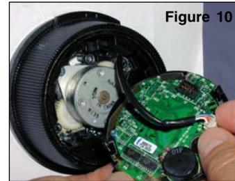
8. Position the generator cable and the ribbon cable around the generator in a counter-clockwise direction to ensure that the cables will not be pinched when you attach the keypad assembly. (Figure 12).
